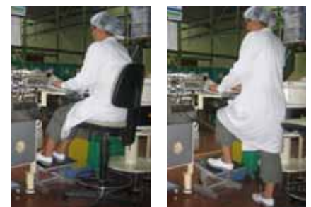
Ergonomic adjustments to condom foiling machines allowing operators to sit or stand, minimising posture-related problems.
